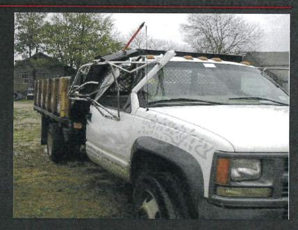
Of course, before products can be delivered, the trucks need to be loaded. As you can see in this picture, someone was not being too careful while using the front end loader, turning this perfectly good vehicle into a perfect total loss.
